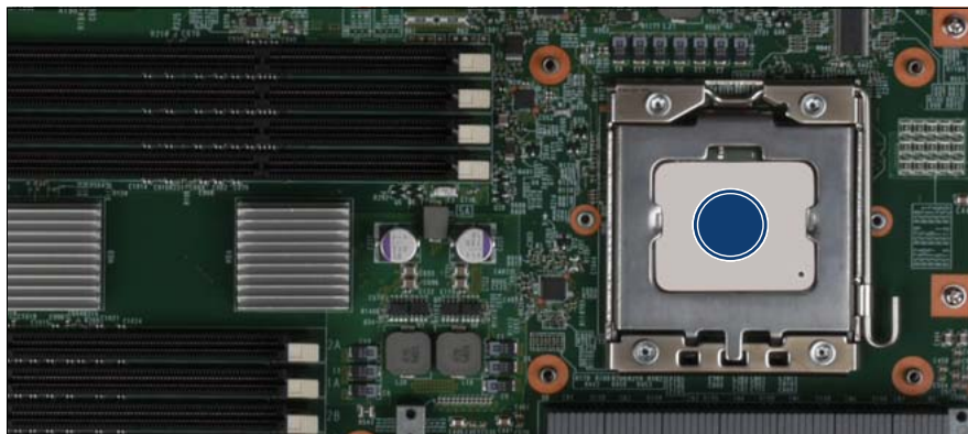
Figure 130: Applying the thermal paste
